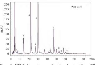
Figure 5. HPLC chromatogram of methanol extract from GT, where 1-GC, 2-Theobromine, 3-EGC, 4-Caffeine, 5-EC, 6-EGCG, 7-ECG, 8-Rutin, 9-Q3G, 10-K3RG.
