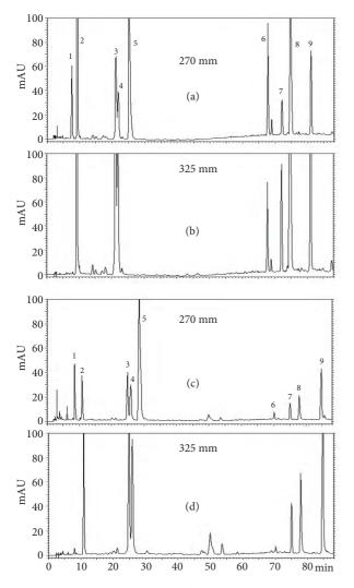
Figure 4. HPLC chromatograms of methanol extracts at 270 and 325 nm from GM (a, b) and RM (c, d), where 1-Theobromine 2-Neochlorogenic acid, 3-Chlorogenic acid, 4-Cryptochlorogenic acid, 5-Caffeine, 6-Rutin, 7, 8 and 9-Unidentified caffeoyl derivatives.
