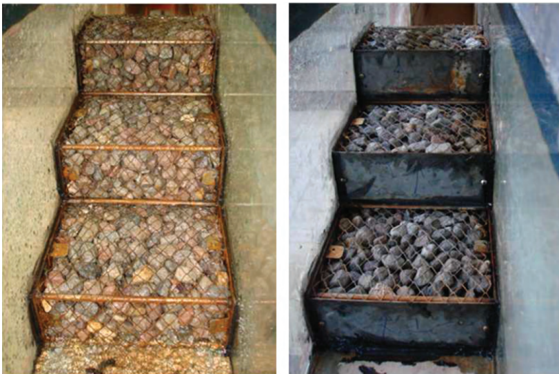
Figure 2. Gabion stepped weirs with a slope of 1:2, without vertical impervious plate (left) and with vertical impervious plate (right).
