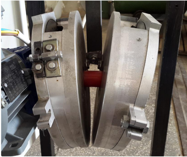
Figure 6. Assembled view of the metering unit with twin vacuum disks.
