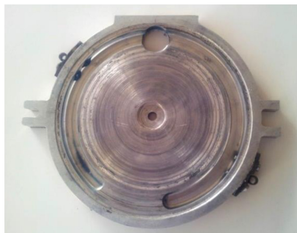
Figure 5. Manufactured view of the lid for right side metering unit in the direction of travel.
