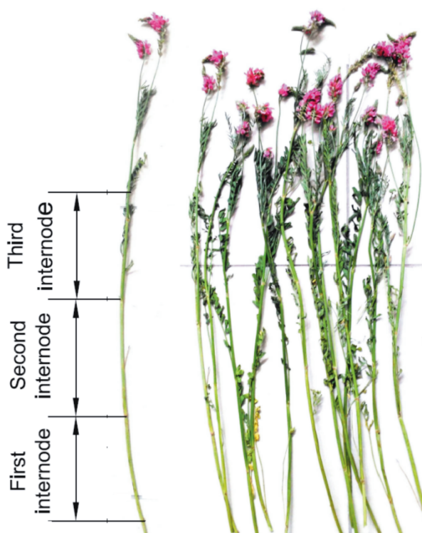
Figure 6. Regions identifying the internodes of the sainfoin stem in the shearing and bending tests.
