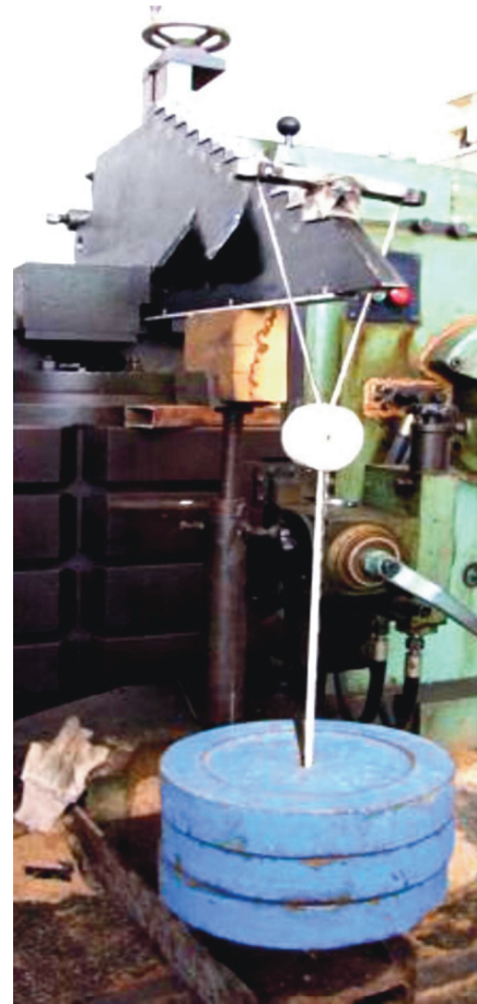
Figure 8. Static calibration tests for force measurement.
