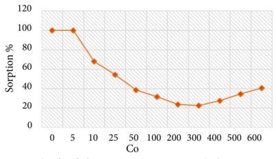
**Figure 6.** The effect of solution concentration on P sorption (Sorbent amount; 1 g / 30 mL, temperature; 21 ± 2 °C, particle size; 0.42 mm, shaking time; 12 h, pH = 6.12)
