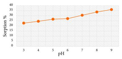
**Figure 3.** The effect of pH on P sorption ( $C_0$ ; 100 mg L<sup>-1</sup>, shaking time; 4 h, amount of sorbent; 1 g / 30 mL, temperature; 21 ± 2 °C, particle size; 0.42 mm)
