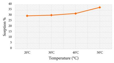
**Figure 4.** The effect of temperature on P sorption ( $C_0$ ; 100 mg L<sup>-1</sup>, shaking time; 4 h, sorbent amount; 1 g / 30 mL, particle size; 0.42 mm, pH = 6.12).
