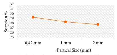
**Figure 2.** The effect of particle size on P sorption ( $C_0$ ; 100 mg L<sup>-1</sup>, shaking time; 4 hours, amount of sorbent; 1 g / 30 mL, temperature; 21 ± 2 °C, pH = 6.12)
