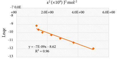
**Figure 8.** Evaluation of P sorption by gyttja with D-R isotherm (Sorbent amount; 1 g / 30 mL, temperature;  $21 \pm 2$  °C, particle size; 0.42 mm, shaking time; 12 h, pH = 6.12)
