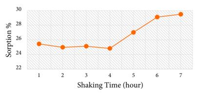
**Figure 5.** The effect of shaking time on P sorption ( $C_0$ ; 100 mg L<sup>-1</sup>, sorbent amount; 1 g / 30 mL, temperature; 21 ± 2 °C, particle size; 0.42 mm, pH = 6.12).
