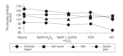
Figure 1. The Effects of Bleaching Chemicals on the Bending Strength of Wood (N/mm<sup>2</sup>).
