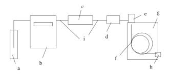
Figure 2. Schematic diagram of on-line SFE-SFC system a)  $CO_2$  cylinder b) pump c) extraction vessel d) cryotrapheater e) injection port f) chromatography column g) column oven h) detector i) transfer lines.
