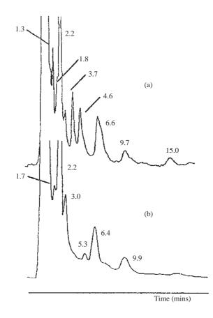
**Figure 3.** Comparison of the HPLC chromatograms of (a) chloroform and (b) supercritical carbon dioxide extracts of feverfew powder (For conditions see text; retention times in minutes).
