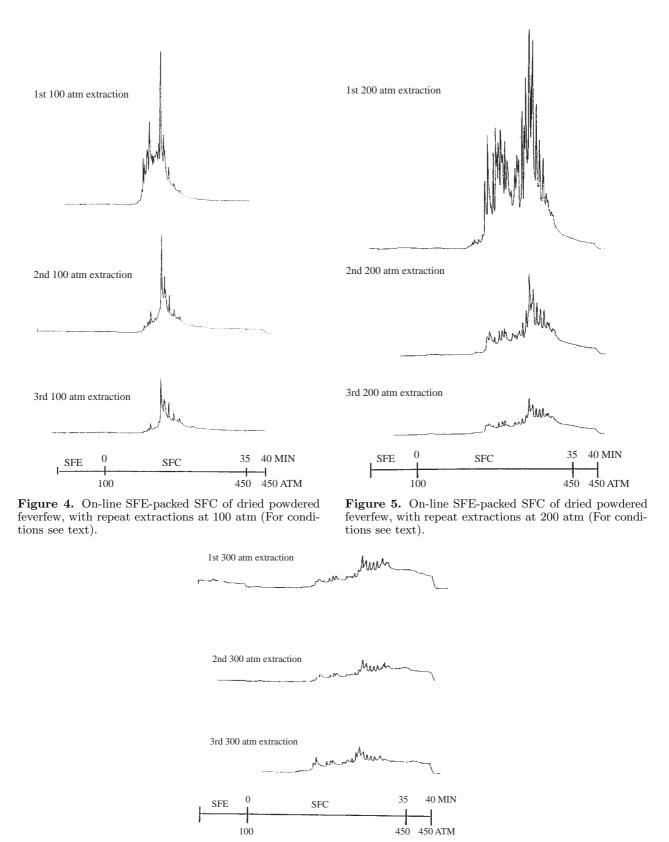
Figure 6. On-line SFE-packed SFC of dried powdered feverfew, with repeat extractions at 300 atm (For conditions see text).
