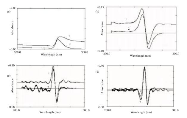
Figure 2. UV-Absorption (a), first derivative (b), second derivative (c), third derivative (d) spectra of green pepper (1) and AA (2) (c = 10  $\mu$ g ml<sup>-1</sup>)
