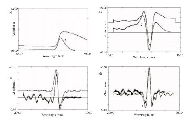
Figure 3. UV-Absorption (a), first derivative (b), second derivative (c), third derivative (d) spectra of chestnut (1) and AA (2) (c = 10  $\mu$ g ml<sup>-1</sup>)
