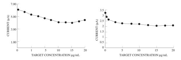
Figure 5. Calibration plots of (A) MB and (B)  $[Ru(bpy)_3]^{2+}$  peak current aganist target concentration. Other conditions are as in Figure 1.
