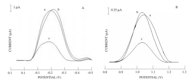
Figure 2. Differential pulse voltammograms for [A] 20  $\mu$ M MB and [B] 20  $\mu$ M [Ru(bpy)<sub>3</sub>]<sup>2+</sup>label at the 17-base *Microcystis* spp. probe (sequence B)-immobilized electrode; (a) before hybridization; (b) after hybridization with the two-bases mismatch oligonucleotide (sequence A'), (c) after hybridization with 17-base *Microcystis* spp. target (sequence A). Other conditions are as in Figure 1.
