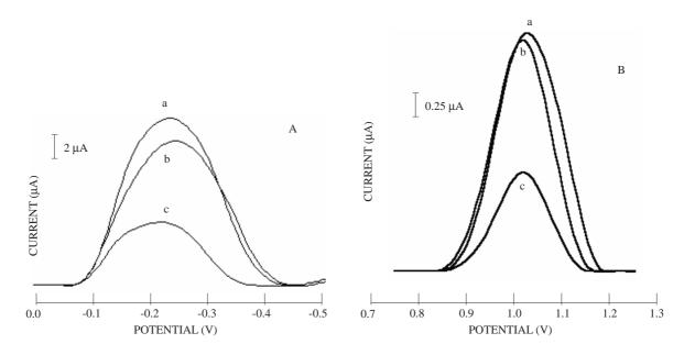
Figure 4. Differential pulse voltammograms for [A] 20  $\mu$ M MB and [B] 20  $\mu$ M [Ru(bpy)<sub>3</sub>]<sup>2+</sup>label at the 17-base *Microcystis* spp. probe (sequence B)-immobilized electrode; (a) before hybridization, (b) after hybridization with the noncomplementary oligonucleotide (sequence C), (c) after hybridization with 17-base *Microcystis* spp. target (sequence A). Measurements of accumulated label in blank TBS by using DPV. Other conditions are as in Figure 1.
