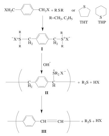
Figure 2. Synthesis and processing scheme of PPV.
