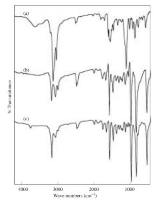
Figure 3. FTIR spectra of (a) the EPPV (b) the EPPV-180 and (c) the EPPV-245 (by using KBr pellet at room temperature).
