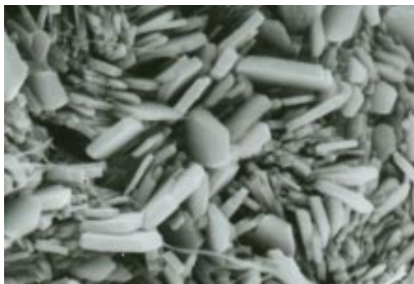
Figure 1. SEM micrograph of raw clinoptilolite-rich tuff from Nižný Hrabovec (East Slovakia); magnification x 3700.
