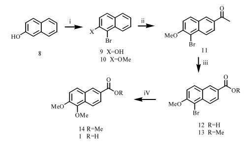
Scheme 2. Reagents and Conditions: (i) a) Br<sub>2</sub>, AcOH, 88% b) Me<sub>2</sub>SO<sub>4</sub>/K<sub>2</sub>CO<sub>3</sub>, acetone, 95% (ii) AcCl /AlCl<sub>3</sub>, 1,2-dichloroethane, 86% (iii) a) Br<sub>2</sub>/NaOH, HCl, 88% b) MeOH/TsOH, 98% (iv) a) NaOMe/MeOH, DMF, CuI b) NaOH/MeOH-H<sub>2</sub>O, then HCl, 82%.
