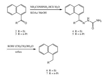
Figure 2. The conversion of ketones 2 and 3 to their respective semicarbazones (4 and 5) followed by reduction to the 1-*n*-alkylnaphthalenes 6 and 7.
