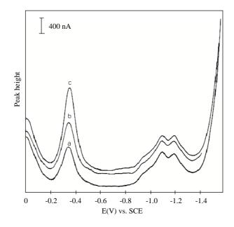
Figure 5. Determination of Cu in cabbage leaf sample: (a) 10 mL sodium acetate, pH 6.5, 1.0 mL 0.1 M EDTA + 0.2 mL sample (b) (a) + 0.1 mL  $10^{-3}$ M Cu(II) (c) (b) + 0.1 mL  $10^{-3}$ M Cu(II).
