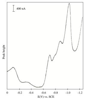
Figure 2. DPP polarogram of cabbage leaf sample: 10 mL 1 M acetate buffer, pH 4, + 0.2 mL digested sample.
