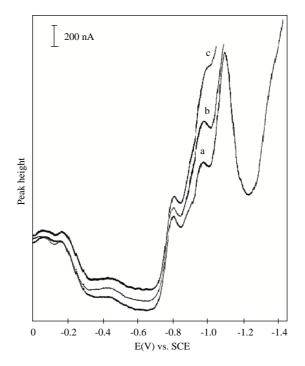
Figure 3. Determination of Cr in cabbage leave sample: (a) 10 mL 1 M acetate buffer, pH 4, + 0.2 mL sample, (b) a + 0.05 mL  $10^{-3}$  M Cr(III), (c) (b) + 0.05 mL  $10^{-3}$ M Cr(III).
