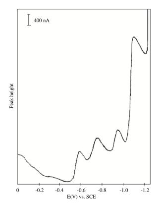
Figure 1. DPP polarogram of cabbage leaf sample: 10 mL 1 M acetic acid, acetate solution, pH 2, +0.2 mL digested sample.
