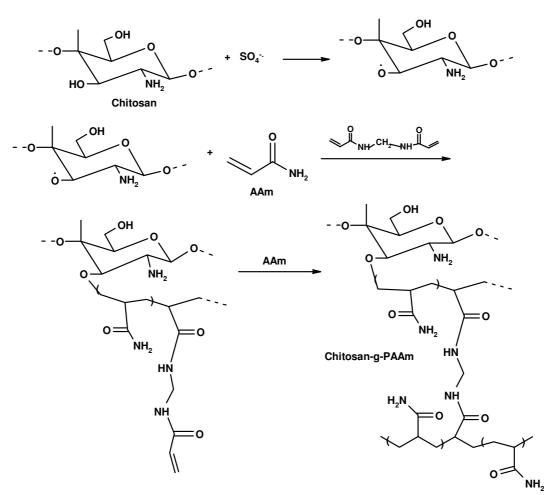
**Scheme.** General mechanism for APS-initiated graft copolymerization of acrylamide onto chitosan in the presence of MBA.
