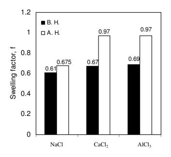
Figure 5. Dependence of the dimensionless salt sensitivity (f) for non-hydrolyzed and hydrolyzed chitosan-g-PAAm hydrogels on the valance of the metal cation (0.15 molar solutions). AH, after hydrolysis; BH, before hydrolysis.
