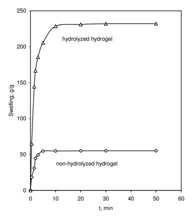
Figure 9. A plot of water content W and time according to Equation 5 (first-order kinetics) for both hydrogels.
