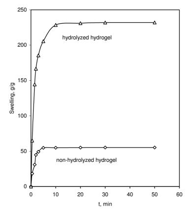
Figure 8. Swelling ratio as a function of time for chitosan-g-PAAm hydrogel before and after hydrolysis.
