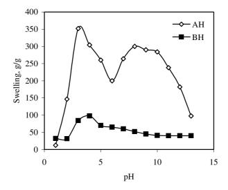
Figure 6. Swelling behavior of chitosan-g-PAAm and H-chitosan-g-PAAm at various pHs. AH, after hydrolysis; BH, before hydrolysis.
