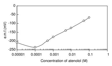
Figure 2. Calibration curve of atenolol selective electrode based on (A-TP) ionophore and DBPH plasticizer.
