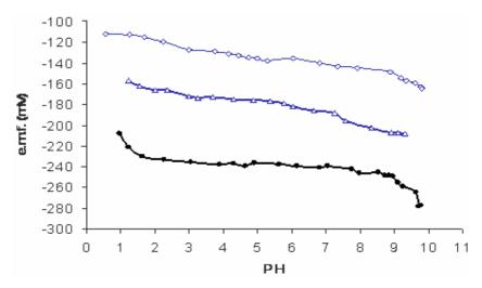
Figure 3. Effect of pH on response of the electrode IV at different atenolol concentrations. o  $-10^{-2}$  M,  $\Delta - 10^{-3}$  M,  $\bullet - 10^{-4}$  M.
