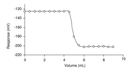
Figure 5. Titration curve for sample solution containing 5 mL of 0.01M atenolol with 0.01 M PT standard solution as titrant.
