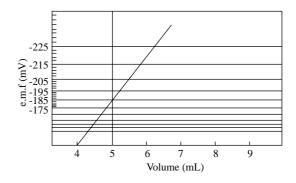
Figure 4. Multi-standard addition method for the determination of 0.01 M atenolol sample using Gran's plot paper with membrane IV.
