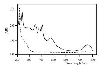
Figure 4. Absorbance spectra of  $2 \times 10^{-4}$  M NH<sub>4</sub>VO<sub>3</sub> solution (- - - -), and  $1 \times 10^{-4}$  M NH<sub>4</sub>VO<sub>3</sub> in the presence of  $2 \times 10^{-4}$  M NA solution (-----).
