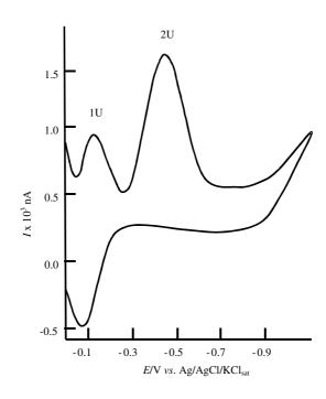
Figure 2. Cyclic voltammogram of  $5 \times 10^{-5}$  M NH<sub>4</sub>VO<sub>3</sub> solution in the phosphate buffer (pH 7.4). 1U: the reduction of V(V) to V(IV); 2U: the reduction of V(IV) to V(III). Experimental conditions: scan rate: 500 mV s<sup>-1</sup>; scan increment: 2 mV; equilibrium time: 5 s; drop size: medium.
