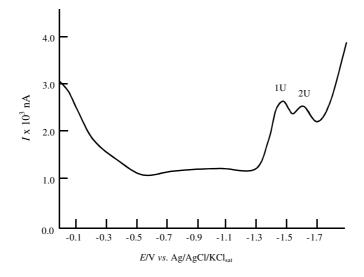
Figure 1. Square-wave voltammogram of  $4.76 \times 10^{-4}$  M NA solution in the phosphate buffer (pH 7.4). 1U: the formation of the aldehyde derivative of NA (-1.48 V); 2U: the formation of the carbinol derivative of NA (-1.61 V). Experimental conditions: scan rate: 200 mV s<sup>-1</sup>; equilibrium time: 5 s; frequency: 100 Hz; drop size: medium.
