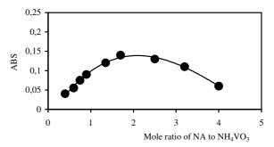
Figure 5. Plot of the absorbance at 415 nm versus the mole ratio of NA to NH<sub>4</sub>VO<sub>3</sub>.
