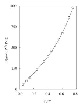
Figure 1. BET plot of nitrogen adsorption on surface area reference material (SARM).
