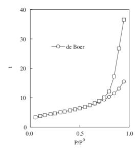
Figure 3. Plot of thickness of adsorbed layer "t" (in Angstrom) as a function of relative pressure "P/P<sup>o</sup>" (thickness data obtained on the basis of Eq. (39) and (41)).
