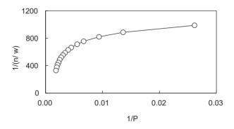
Figure 2. Langmuir plot of nitrogen adsorption on SARM.
