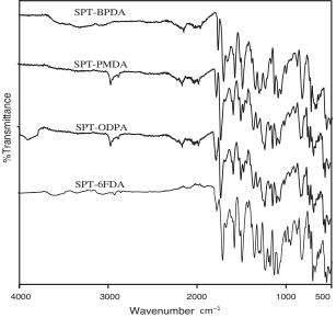
Figure 4. FTIR spectra of PTSIs.
