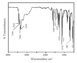
Figure 1. FTIR spectrum of SPT.
