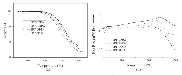
Figure 6. TGA curves of PTSIs obtained at heating rate of 10  $^{\circ}$ C min<sup>-1</sup> in an inert atmosphere of nitrogen (a). DSC thermograms of PTSIs obtained at a heating rate of 10  $^{\circ}$ C min<sup>-1</sup> under nitrogen flow (b).
