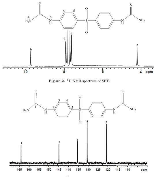
Figure 3. <sup>13</sup>C NMR spectrum of SPT.
