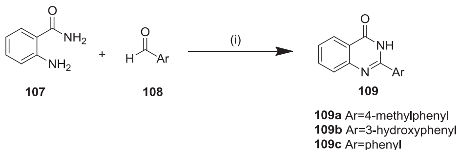
Scheme 25. Synthesis of 2-arylquinazolin-4(3H)-ones 109a , 109b , and 109c . Reagents and conditions: (i) CuCl 2 ·2H 2 O, EtOH, reflux.
