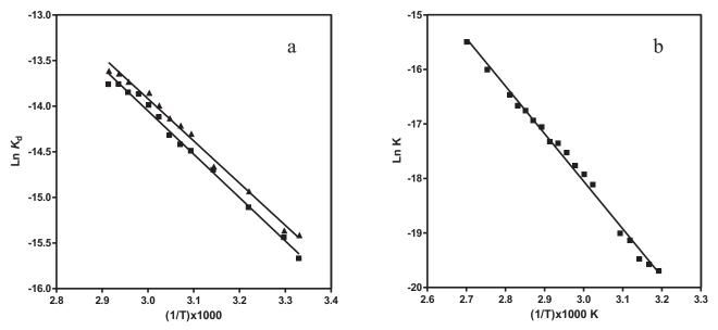
Figure 10. Plots of  $\ln K_d$  versus 1/T for the gelators: (a) 1 in CD<sub>3</sub>CN and (b) 4 in d<sub>8</sub>-toluene at 25 °C.
