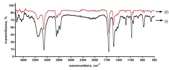
Figure 6. FTIR spectra of 4 in the solid state and the xerogel form from xylene gel.
