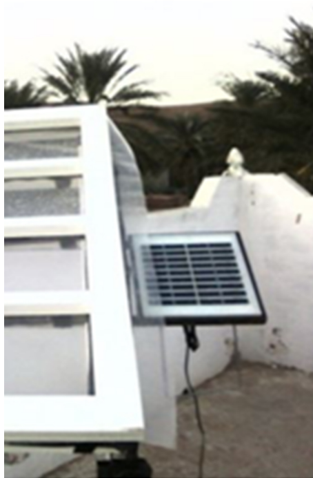
Figure 11. Solar cells (right) for the energy measurement during natural weathering.
