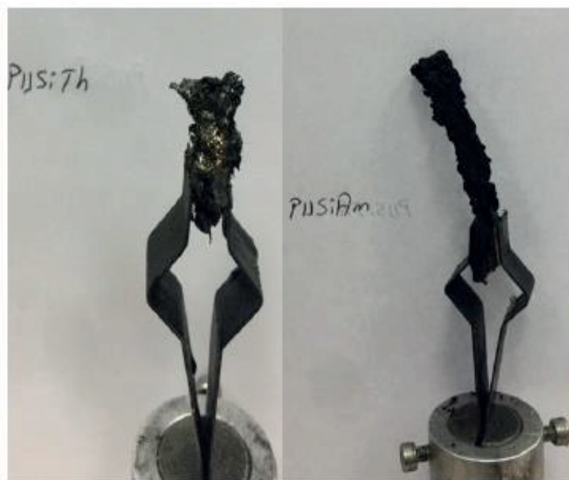
Figure 12. Photographs of char residues from (a) PUSiTh, (b) PUSiAm after LOI test
