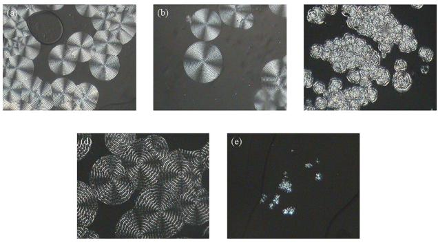
**Figure 1.** Polarized optical micrographs of PPDO spherulites after isothermal crystallization at different temperatures (*Tc*) for different time (*tc*): (a) Tc = 60 °C, tc = 6 min, (b) Tc = 70 °C, tc = 19 min, (c) Tc = 80 °C, tc = 30 min, (d) Tc = 90 °C, tc = 110 min, (e) Tc = 100 °C, tc = 100 min.
