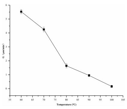
**Figure 2.** Radius growth rate of spherulites (G) of PPDO as a function of crystallization temperature (*Tc*).
