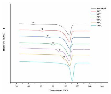
Figure 5. DSC thermograms of PPDO after isothermal annealing at various Ta for 2 h.
