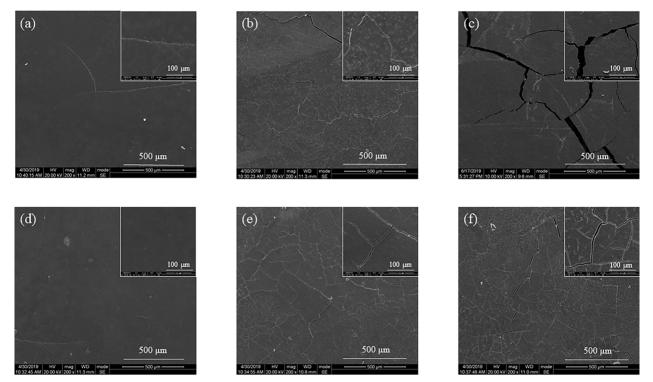
**Figure 11.** SEM micrographs of PPDO bars after degradation: (a) untreated PPDO for 2 weeks, (b) untreated PPDO for 4 weeks, (c) untreated PPDO for 5 weeks, (d) annealed PPDO for 2 weeks, (e) annealed PPDO for 4 weeks (f) annealed PPDO for 5 weeks.
