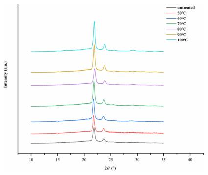
**Figure 8.** WAXD of PPDO in the range of  $10 \sim 35^{\circ}$  (2-theta) after isothermal annealing at various *Ta* for 2 h.
