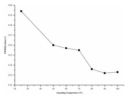
**Figure 10.** Changes in FWHM of X-ray diffraction peak (21.90°) after isothermal annealing at various *Ta* for 2 h.
