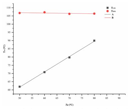
**Figure 6.** Peak melting temperatures of PPDO as a function of *Ta* after isothermal annealing for 2 h: (A) linearly fitting of  $T_{LM}$  (B) linearly fitting of  $T_{HM}$ .
