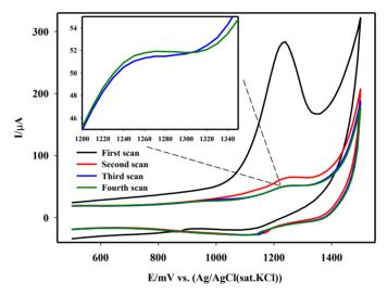
Figure 1. Cyclic voltammograms of 5  $\times$  10<sup>-5</sup> M spiramycin on MWCNTs-COOH/GCE.
