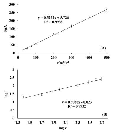
**Figure 6.** The plots of (A) *I* vs.  $\nu$  and (B) log *I* vs. log  $\nu$  for the oxidation of spiramycin at scan rates of 25, 50, 75, 100, 200, 300, 400, and 500 mV s<sup>-1</sup> on MWCNTs-COOH/GCE
