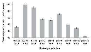
**Figure 3.** Percentages of the maximum anodic peak current of  $5 \times 10^{-5}$  M spiramycin obtained by cyclic voltammetry in different electrolyte solutions on MWCNTs-COOH/GCE with stirring the electrolyte solution at 300 rpm for 60 s. NAS, nitric acid solution; PBS, phosphate buffer solution.
