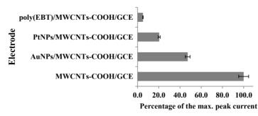
**Figure 7.** Percentages of the maximum anodic peak current of  $5 \times 10^{-5}$  M spiramycin obtained by cyclic voltammetry on different electrode surfaces with stirring the electrolyte solution at 300 rpm for 60 s.
