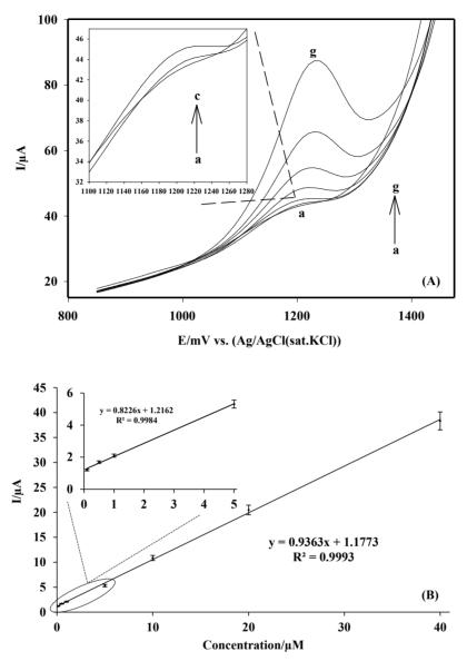
**Figure 8.** (A) Linear sweep voltammograms of serial standard solutions of spiramycin in 0.2 M HNO3 with stirring the electrolyte solution for 60 s on MWCNTs-COOH/GCE; (a–g): 0.100, 0.500, 1.00, 5.00, 10.00, 20.00, and 40.00  $\mu$ M. (B) The calibration graph.
