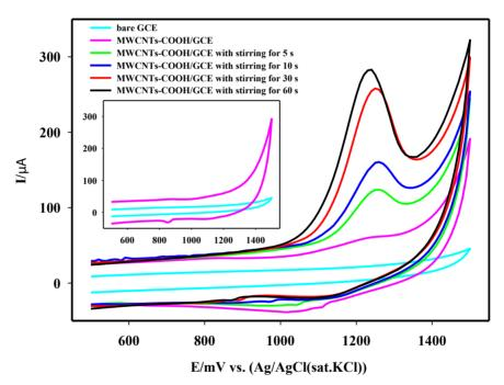
**Figure 4B.** Cyclic voltammograms of  $5 \times 10^{-5}$  M spiramycin in 0.2 M HNO<sub>3</sub>. Inset showed background cyclic voltammograms.
