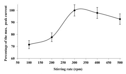
**Figure 5.** The influence of stirring rate between 100 and 500 rpm on the oxidation peak current of  $5 \times 10^{-5}$  M spiramycin in 0.2 M HNO<sub>3</sub> solution.
