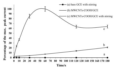
**Figure 4A.** Percentages of the maximum anodic peak current of  $5 \times 10^{-5}$  M spiramycin obtained by cyclic voltammetry on (a) bare GCE with stirring the electrolyte solution, (b) MWCNTs-COOH/GCE, (c) MWCNTs-COOH/GCE with stirring the electrolyte solution.
