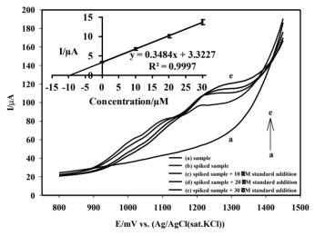
**Figure 9.** Linear sweep voltammograms of (a) sample, (b) spiked sample, and after addition of (c) 10.00  $\mu$ M, (d) 20.00  $\mu$ M, and (e) 30.00  $\mu$ M spiramycin standard. The standard addition calibration graph is given inset.
