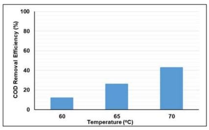
Figure 13. Effect of temperature on COD removal efficiencies (COD/S<sub>2</sub>O<sub>8</sub> = 1/2).
