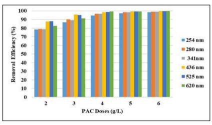
Figure 3. Effect of adsorbent doses on UV-vis absorbance values removal efficiencies.
