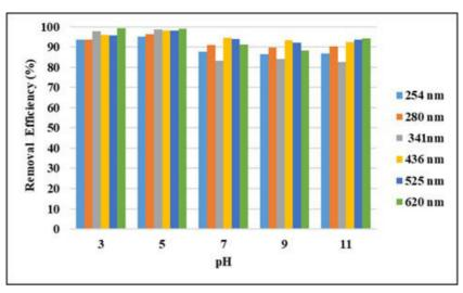
**Figure 1.** pH effect on UV-vis absorbance values removal efficiencies (PAC dose: 4 g/L, contact time: 2 h).
