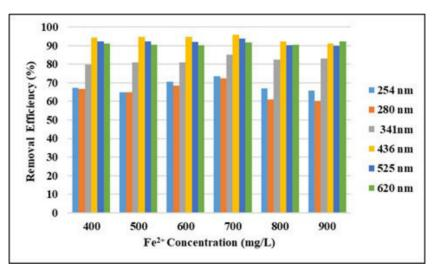
**Figure 10.** Effect of Fe<sup>2+</sup> concentration on COD removal efficiencies (pH: 3,  $H_2O_2$ : 3000 mg/L).
