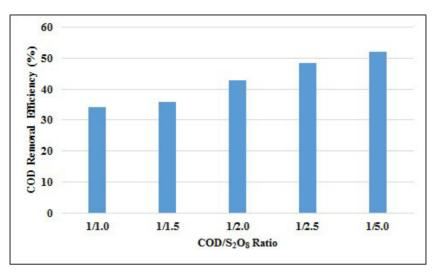
Figure 15. Effect of COD/S<sub>2</sub>O<sub>8</sub> ratio on COD removal efficiencies (T:70 °C, t: 5.5 h).
