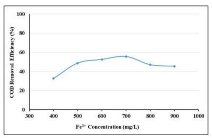
**Figure 9.** Effect of Fe<sup>2+</sup> concentration on removal efficiencies of UV-vis absorbance values (pH: 3, H,O,: 3000 mg/L).
