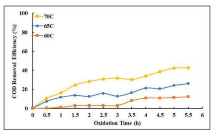
Figure 11. Effect of oxidation time and temperature on COD removal efficiencies  $(COD/S_2O_s = 1/2)$ .
