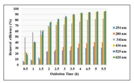
Figure 16. Effect of ozonation on UV-vis absorbance values removal efficiencies.
