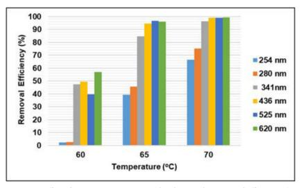
**Figure 12.** Effect of temperature on UV-VIS absorbance values removal efficiencies (t = 5.5 h).
