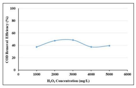
**Figure 8.** Effect of  $H_2O_2$  concentration on COD removal efficiencies (pH: 3, Fe<sup>2+</sup>: 500 mg/L).
