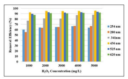
**Figure 7.** Effect of  $H_2O_2$  concentration on removal efficiencies of UV-vis absorbance values (pH: 3, Fe<sup>2+</sup>: 500 mg/L).
