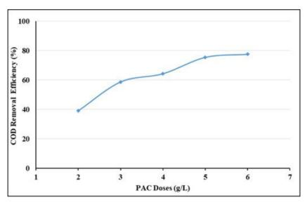
Figure 4. Effect of adsorbent doses on COD removal efficiencies.
