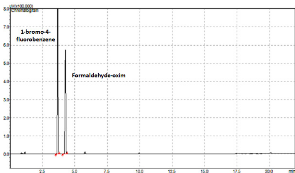
Figure 6. GC-FID chromatogram of 1-bromo-4-fluorobenzene and formaldehyde-oxime.
