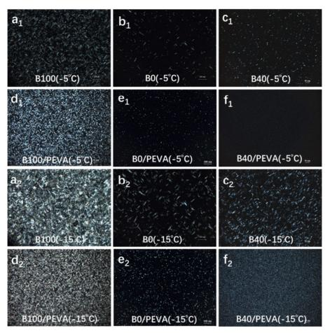
**Figure 3.** POM images of crystal morphologies of B100( $\mathbf{a}_1$  and  $\mathbf{a}_2$ ), B0( $\mathbf{b}_1$  and  $\mathbf{b}_2$ ), and B40( $\mathbf{c}_1$  and  $\mathbf{c}_2$ ) at -5 °C and -15 °C, 1% PEVA treated B100( $\mathbf{d}_1$  and  $\mathbf{d}_2$ ), B0( $\mathbf{e}_1$  and  $\mathbf{e}_2$ ), and B40( $\mathbf{f}_1$  and  $\mathbf{f}_2$ ) at -5 °C and -15 °C.
