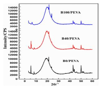
Figure 4. Low-temperature XRD curves of 1wt.% PEVA treated B0, B40, and B100 at -10 °C.
