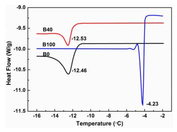
Figure 2. DSC curves of B0, B40, and B100 with 1wt.% PEVA.
