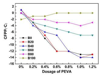
Figure 1. Effect of PEVA on the CFPP of soybean biodiesel blends.
