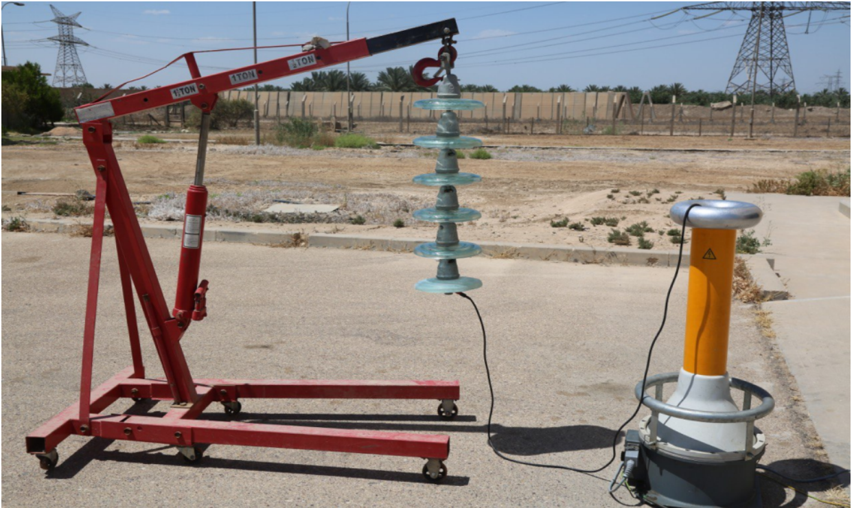
Figure S1. Performance of the high-voltage glass insulator flashover subjected to fast transient overvoltages test
