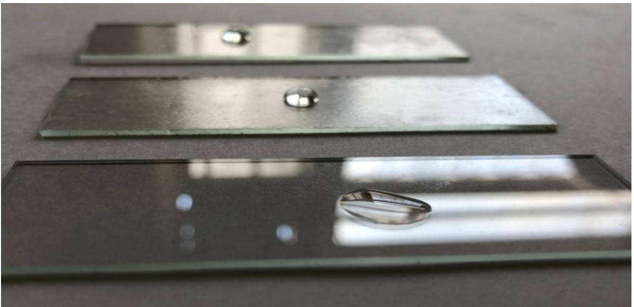
Figure S2. Water contact angles on the natural glass (no coating), glass coating with RTV silicon rubber & RTV silicon rubber/33% nanosilica.
