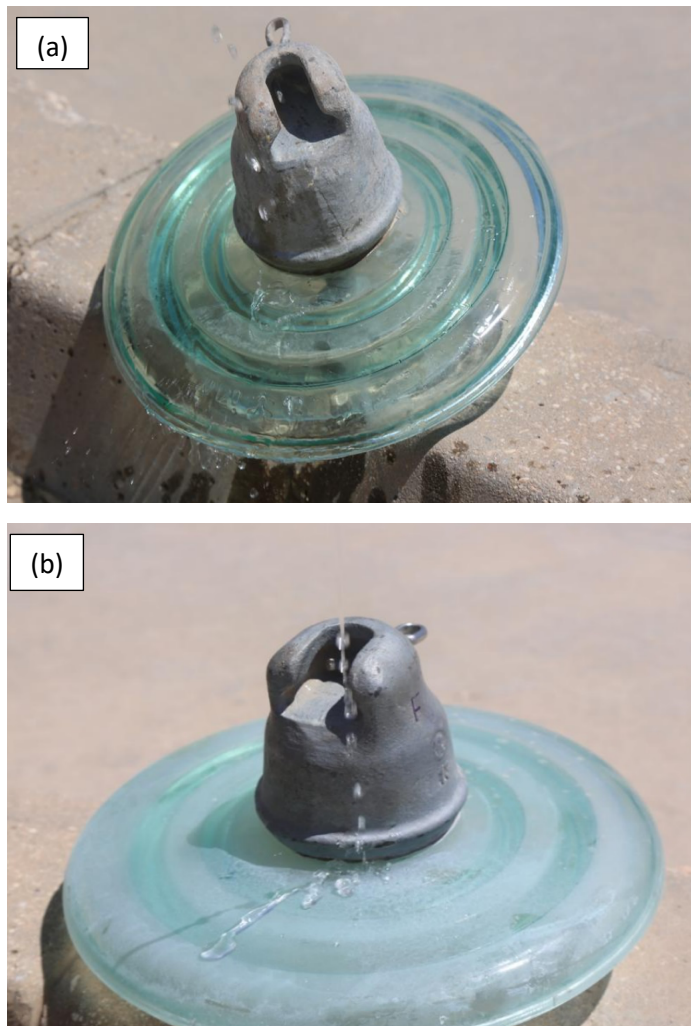
Figure S4. High-voltage glass insulator (a) No coating (pristine glass insulator) (b) Coating with RTV silicon rubber/33% nanosilica
