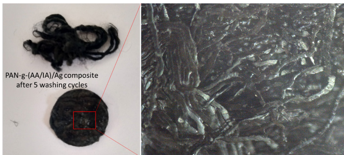
Figure S2. The photograph and optical microscope image of a PAN-g-(AA/IA)/Ag composite fiber after five washing cycles.
