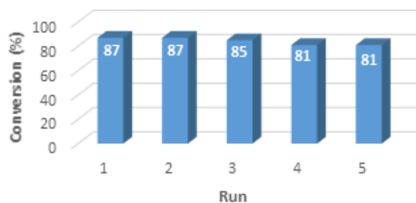
Figure 3. Catalyst reuse; reaction conditions: 1a (0.25 mmol), nitromethane (0.75 mmol), [poly(EGDMA-MATrp)] microbeads (5 mg), MeOH:H 2 O (5:1) (1 mL).
