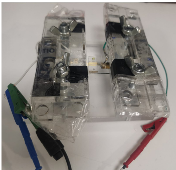
Figure 4. Image of the holder used for stabilization and connection of the integrated devices for electrochemical measurements.
