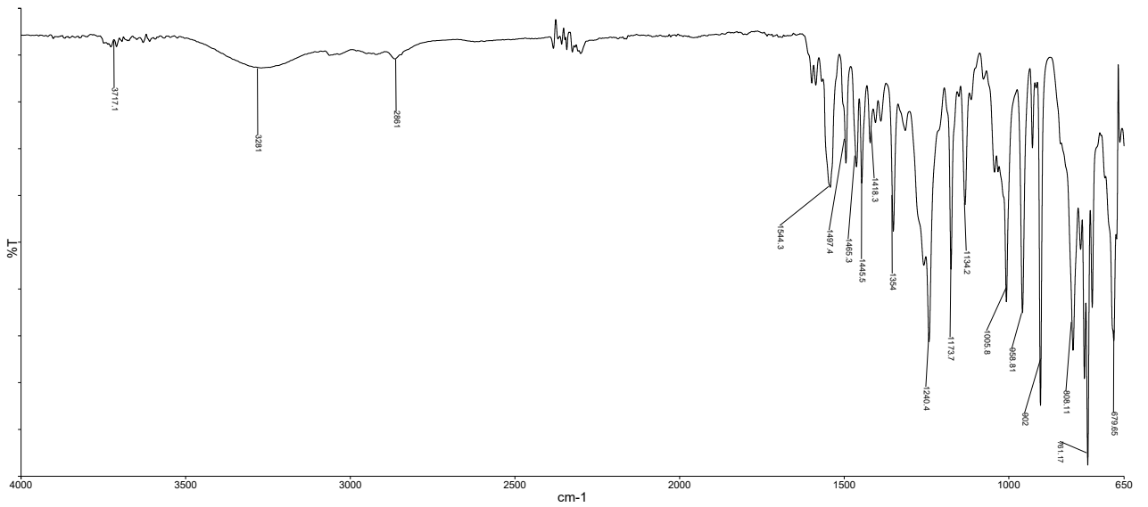
Figure S6. FTIR spectrum of H1.
