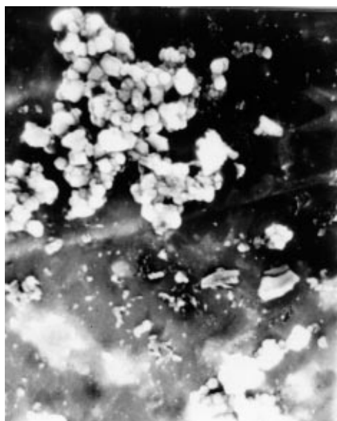
Figure 3. SEM micrograph of poly(p-bromoaniline). (Magnification 800X).
