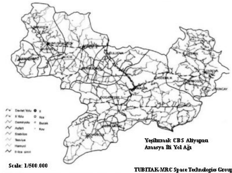
Figure 5. Up-to-date Amasya Province Road Network as extracted from 6 m resolution IRS Pan satellite image.
