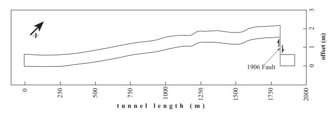
Figure 1. Plan of the Wrights tunnel offset by the 1906 San Francisco earthquake based on a 1908 geodetic survey. The pattern of the tunnel deformation and an elastic dislocation analysis indicate that a second surface rupture observed above the tunnel reflected only secondary effects (after Prentice & Ponti 1997).
