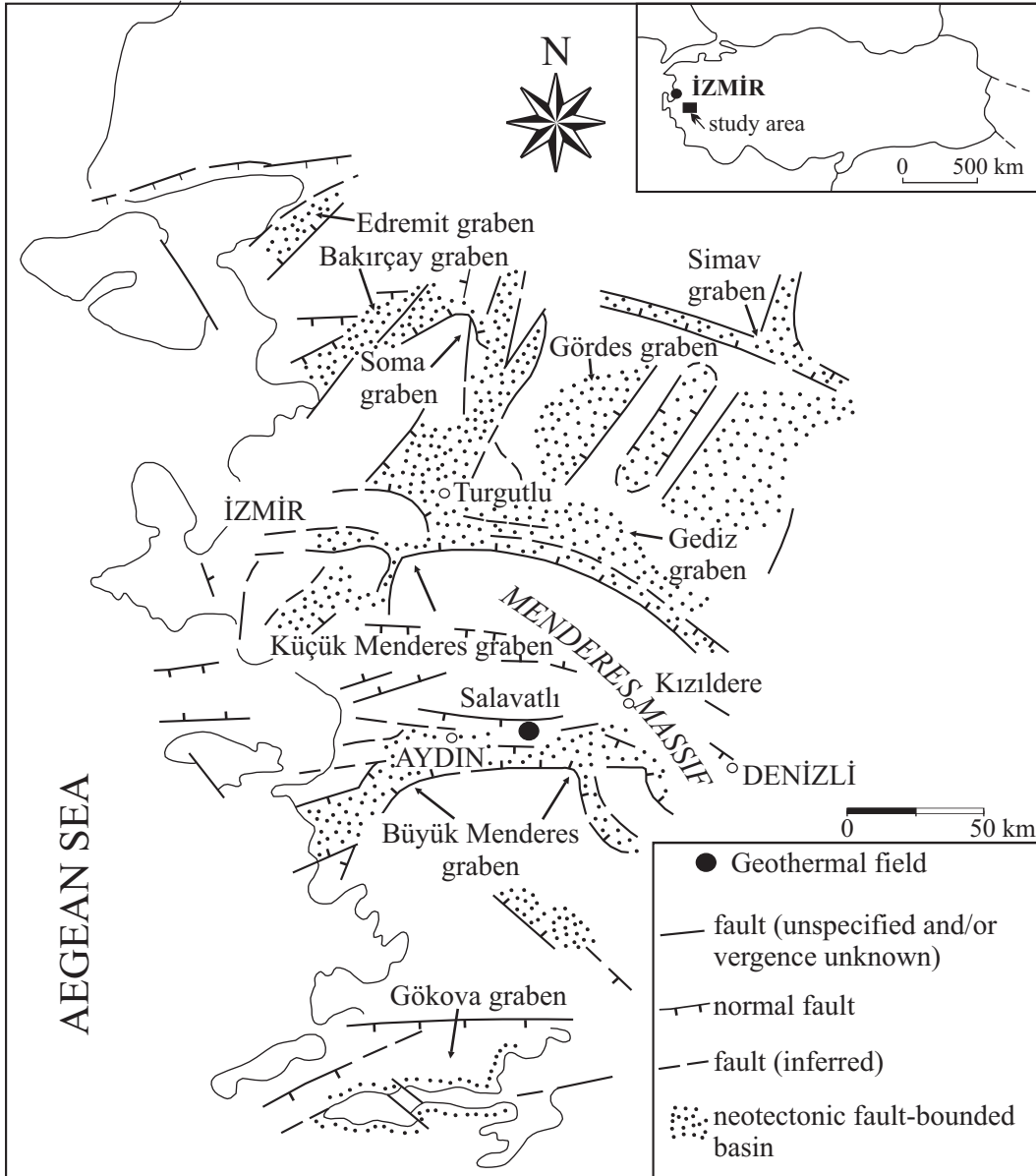
Figure 1. Main tectonic features of western Anatolia and location map of the Aydın-Salavatlı geothermal field.
