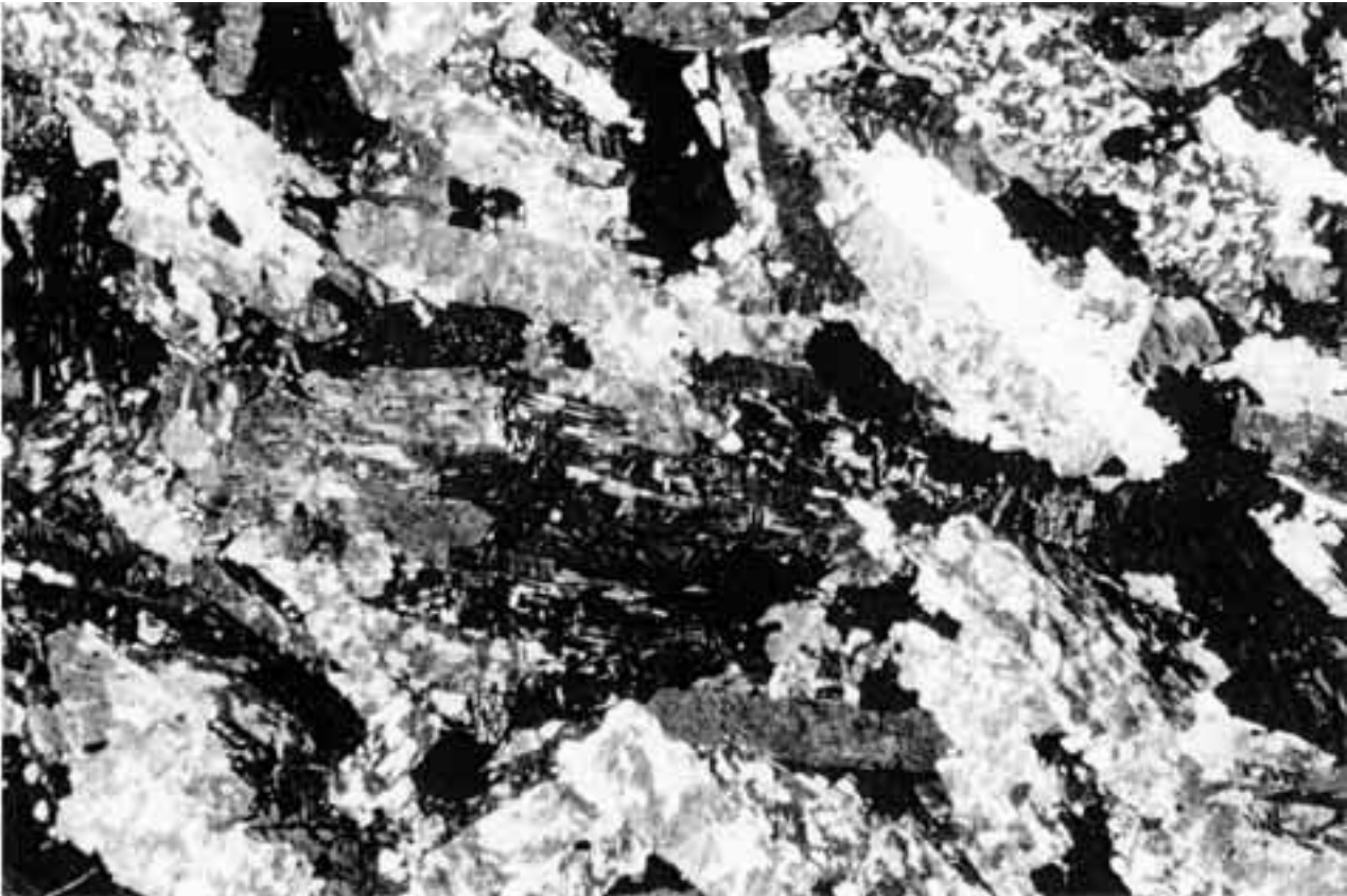
Figure 5. Photomicrograph of tabular alkali feldspars in the alkali-feldspar syenite (sample N40) show strong microperthitic texture. Alkali feldspars also display typical simple twinning. Magnification: 6x3.7 mm, XPL.
