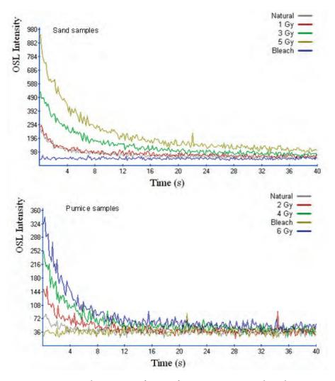
**Figure 3.** OSL decay curves of quartz from representative sandy and pumice samples. OSL signals were recorded from natural, bleached and irradiated aliquots; 1 Gy, 3 Gy and 5 Gy for sand samples and 2 Gy, 4 Gy and 6 Gy for pumice samples.
