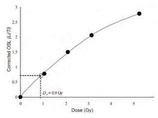
**Figure 2.** Dose-response curve of quartz extracted from sample PRF3-3 can be described by an exponential function for a dose range from 0 to 5 Gy. The equivalent dose is found from corrected natural OSL signal  $(L_n/T_n)$ .
