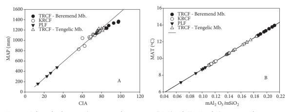
**Figure 5.** Relationship between A) mean annual precipitation (MAP) and CIA–K and B) mean annual temperature (MAT) and the molecular weathering ratio of Al<sub>2</sub>O<sub>3</sub> and SiO<sub>2</sub> in the red clays, palaeosols, and loess deposits.
