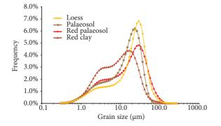
**Figure 3.** Grain-size distribution curves of the red clay (TRCF), red palaeosol (KRCF), and Quaternary loess and palaeosol (PLF) samples from Hungary.
