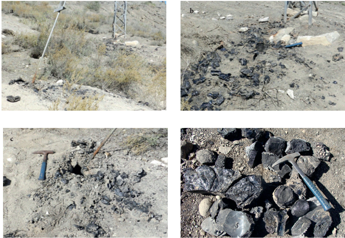
Figure 3. (a) View of the site of the second melting event showing the steel pylon and its support wire; black fragments of glassy material produced during the event may be seen near the base of these structures, (b) close-up view of the products of the second event near the base of the relevant steel pylon (seen in background), (c) another close-up view of basaltic products of the second melting event, scattered around the base of the steel support wire, (d) close-up view of collected samples of basaltic glass associated with the second melting event.
