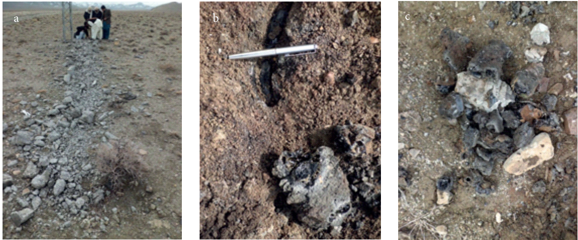
Figure 4. (a) View of the third melting event of 12 February 2011 near the base of another steel pylon of the electric transmission line at Jang Tor Ghar, Muslim Bagh, (b) close-up view near the base of steel pylon of the electric transmission line, (c) close-up view of collected samples of basaltic glass associated with the third melting event.
