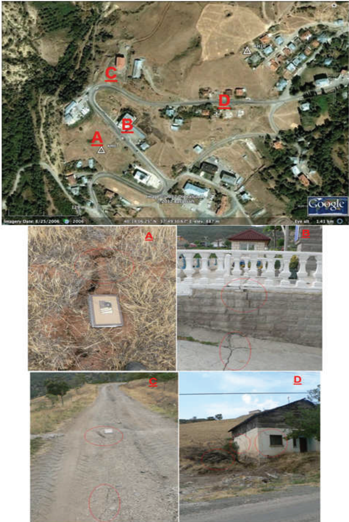
Figure 8. The deformation near KH07 caused fractures and cracks in the buildings and on the ground ( 40^{\circ}18'06''\text{N} , 37^{\circ}49'30''\text{E} ).
