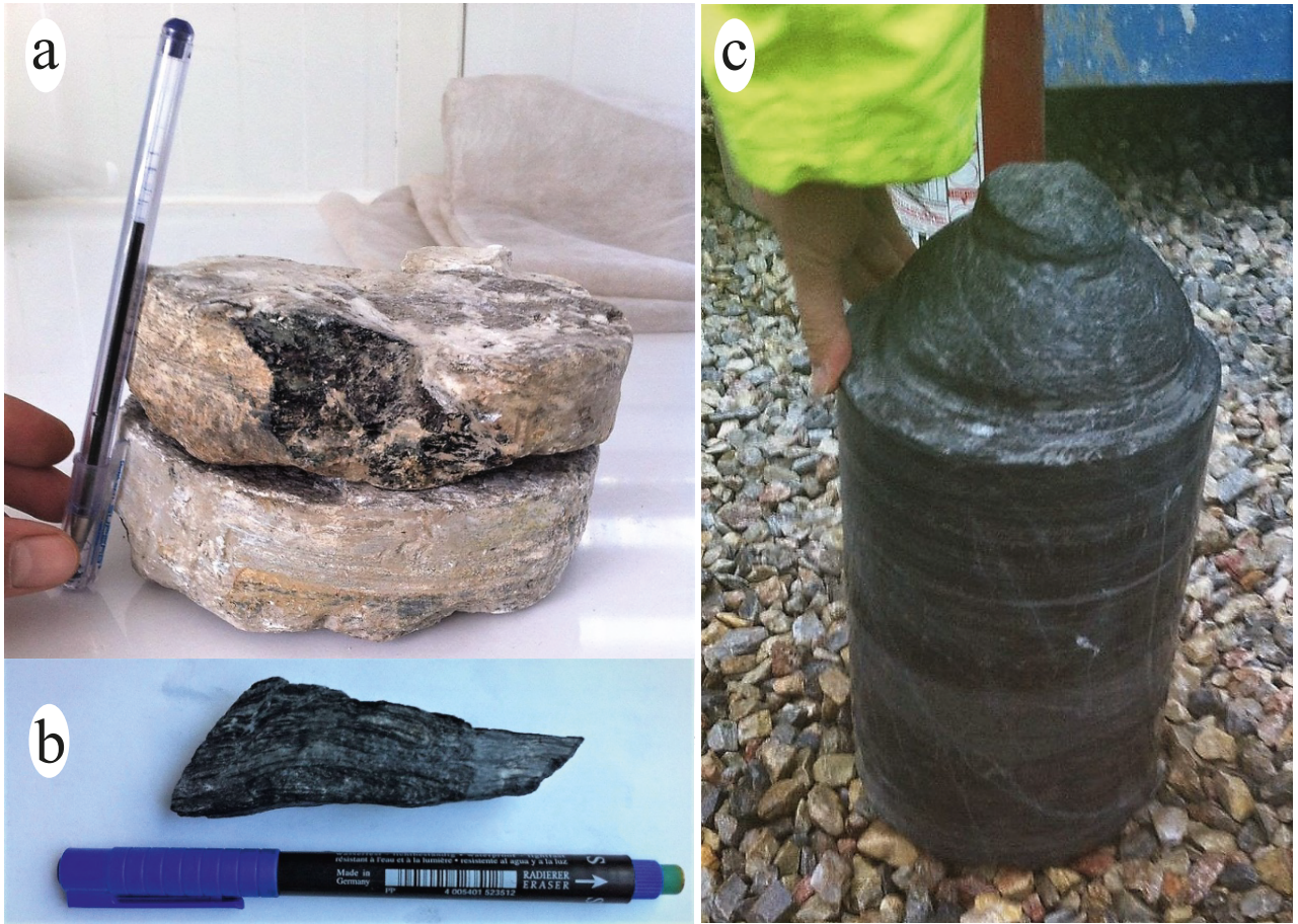
Figure 7. Various samples from the wellbores a) graphite-bearing marble core from Sy-2 well (~1200 m), b) metaquartzite hand specimen from well Sy-13 (1264 m) with well-developed foliation, c) graphite metaquartzite core from Sy-24 well (1080 m).
