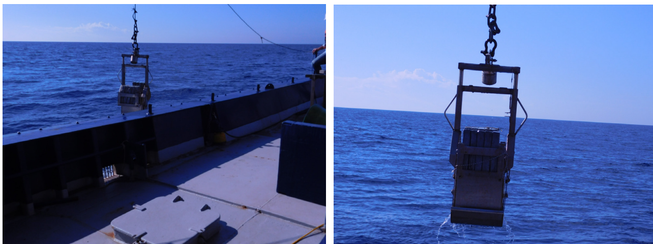
Figure 2. Boxcorer equipment used for the surficial sediment samples (photo taken during sediment sampling for this project).
