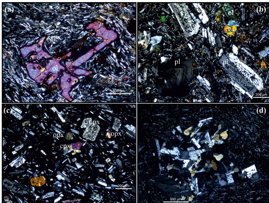
Figure 5. Representative petrographic features of Cumaçay volcanics. a) Skeletal olivine ( ol ) in basalt. b) oscillatory zoned and sieve textured plagioclases ( pl ) in basaltic andesite. c) Orthopyroxene ( opx ) and clinopyroxene ( cpx ) phenocrysts in dacite. d) Pyroxene, plagioclase, and Fe-Ti oxide bearing crystal clots in andesite.
