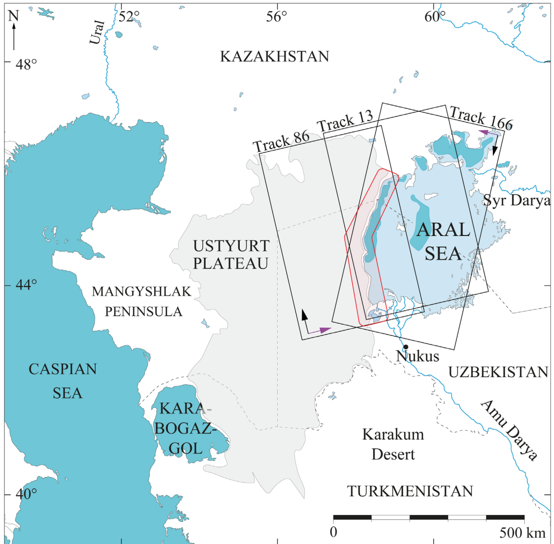
Figure 2. Map of the Aral Sea region showing the geographic position of the Ustyurt Plateau and Sentinel-1 A/B SAR data coverage used in the present study overlain plateau's eastern cliff near the western coast of the Aral Sea. Rectangles labelled with track numbers (aAscending tracks 86 and 13 and descending track 166) indicate the coverage of the IW SAR images. Magenta and black arrows indicate the satellite's LOS look and flight directions, respectively, and the red shaded polygon indicates the selected study area shown in Figure 3.
