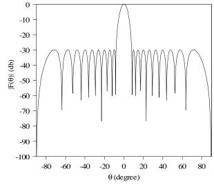
Figure 1. The initial 30-dB Chebyshev pattern
