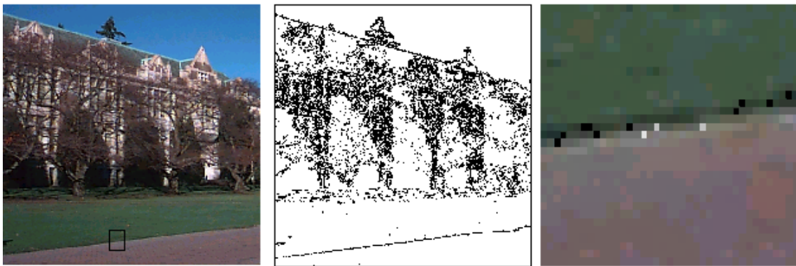
Figure 11. Edge detection and “noise pixels” around an edge
