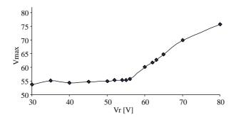
Figure 9. Maximum rail voltage vs. voltage threshold of RPCDs (Vr) for  $R_G = 0.1 \Omega$  for the simulation study case.
