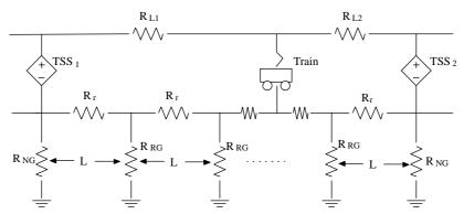
Figure 1. A simple model that can be used for computer simulations of stray currents.
