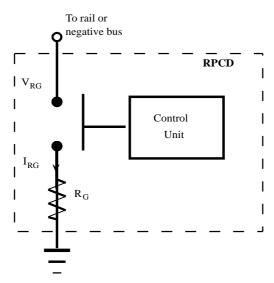
Figure 6. Schematic diagram of the RPCD.
