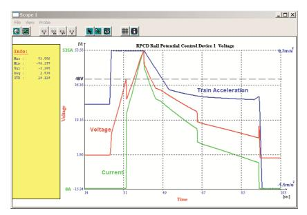
Figure 8. Change in voltage and current on RPCD1 during the acceleration period of the train for  $V_r = 40 \text{ V}$ .
